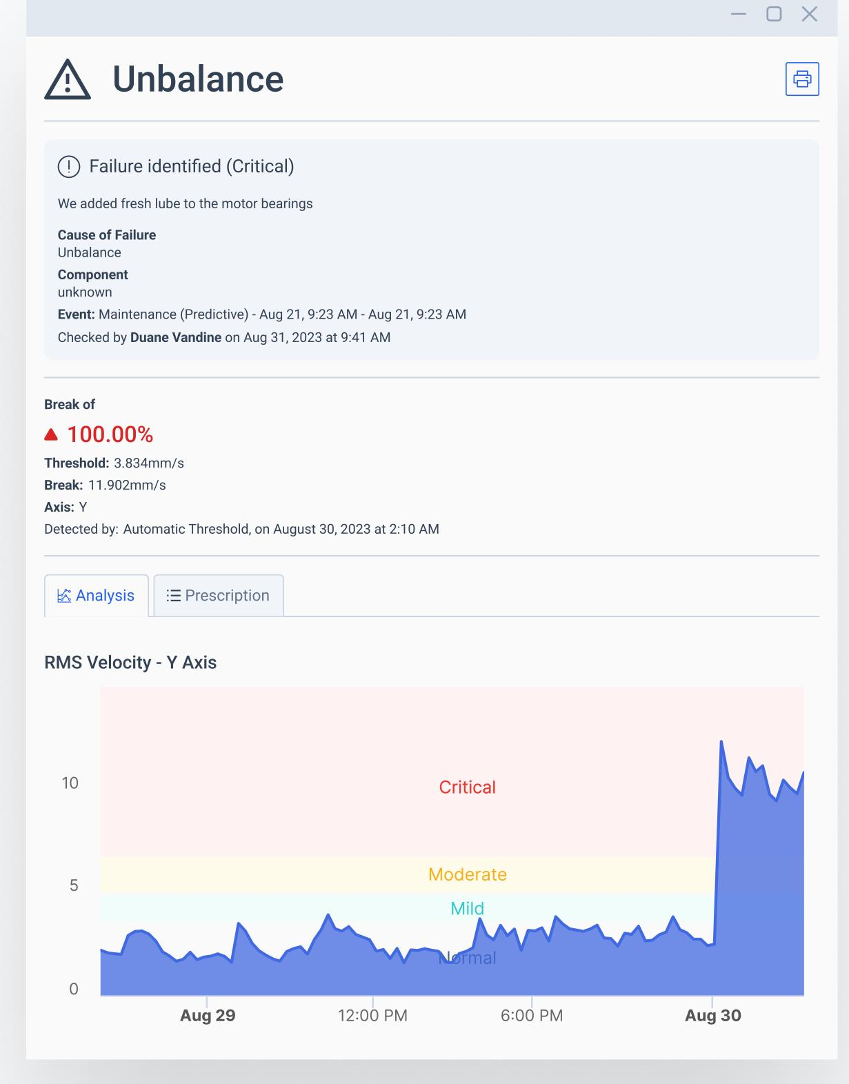
At SWARCO, if one asset goes down, it could cause a complete line stop. TRACTIAN was able to catch this unbalance and let the SWARCO team know ahead of a failure. The condition-based monitoring solution also provided possible causes and a detailed guide of instructions on what to inspect to resolve the unbalance.
